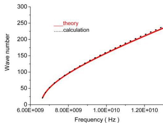
Figure 3. Comparison between theory and calculation of the wave numbers of waveguide TE<sub>10</sub> mode.
